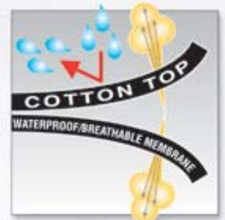
Fabric protector cotton top repels liquids and waterproof/breathable membrane allows body vapor to pass, but not fluids.
